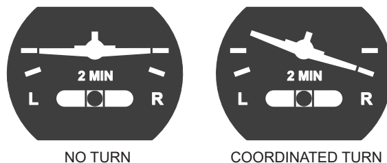
Figure 1.3, Turn Coordinator Needle Positions
